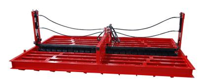
The cutting depth for most standardbred race tracks is 1/8"-1/2'. The 8" inch Tungsten Carbide tipped teeth are easy to replace and adjust with wear and are backed with a 4" welded steel gusset which supports the tooth for added stability. As all Larcom and Mitchell equipment, the cutting depths are easy to adjust and control to the exact preset depths suited for your specific conditions.
