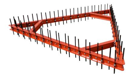
The Larcom and Mitchell 9' Triangle Drag Harrow is the most economical means to condition your soil surface. The double punched I-beams lock in the carbide tipped teeth which can be adjusted as the teeth wear. One of the original designs used back in 1952, Triangle Harrow is a low cost pull behind drag that continues to find a home on Standardbred tracks. All that is required is to hook the drag to the tractor drawbar and go! The 9ft I-Beam Frame has 75 teeth that cut into the racing surface.
